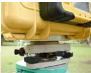
Mounted on Optional Tribrach and adaptor
